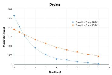
Moisture content of less than 0.025% (250 ppm) is recommended to prevent loss of mechanical properties.
