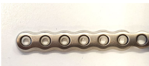
Figure 2. Commercial titanium metacarpal plate on top of the bioresorbable X3 fiber composite plate.
