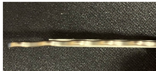
Figure 3. Bioresorbable X3 fiber composite plate behind the commercial titanium metacarpal plate, view from the side.
