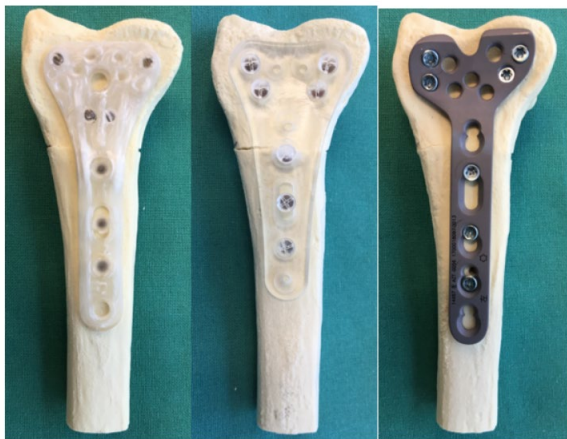
Figure 1. The AFP Radius plate on the left, Commercial Bioabsorbable Radius Plate in the middle and Commercial Titanium Radius plate on the right. Note: figures taken on already tested samples.
